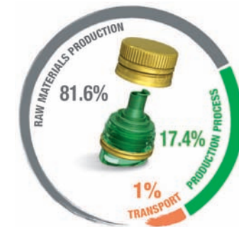
2014 Diagram depicting the % CO 2 equivalent contribution of an oil closure (Source: LCEngineering 2014)
